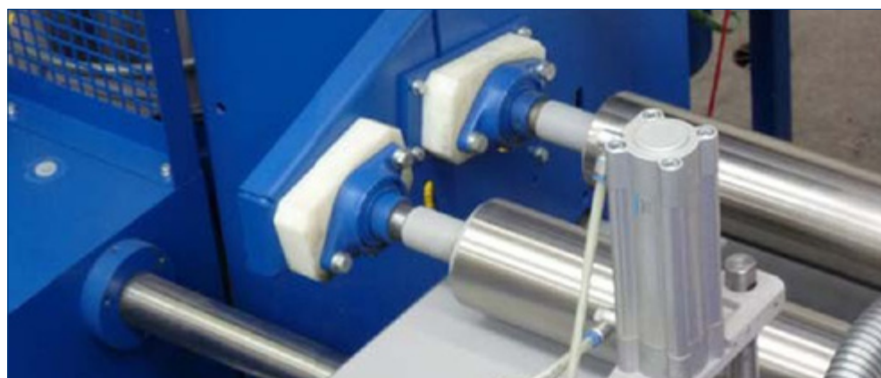
Sensor type RR W to measure over the full fabric width on two rollers
