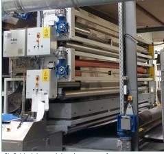
SL C: Modular straightening system for carpets
