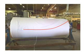
The loss of production until then was about 30%, caused by the wrong straightening of the fabric. Thus, almost all goods had to be straightened manually.
