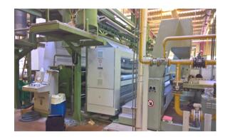
After the start up of the PLEVA straightening machine, all fabrics can now run in automatic mode.
